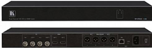
VP-475UX is a high-performance, dual channel scaler and format converter for SDI video signals of up to 12G data rate. With its integrated dual scaler, it converts the 12G SDI video signals from its two input channels (with embedded audio) to two 4K@60Hz (4:4:4) HDMI outputs, along with de-embedding the audio signals and sending them to the analog audio output ports
